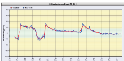
Single point settlement and uplift after mechanical track alignments on the dam.
