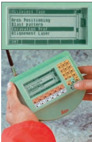
Extremely simple user menu guidance on the RCS1100 remote control
