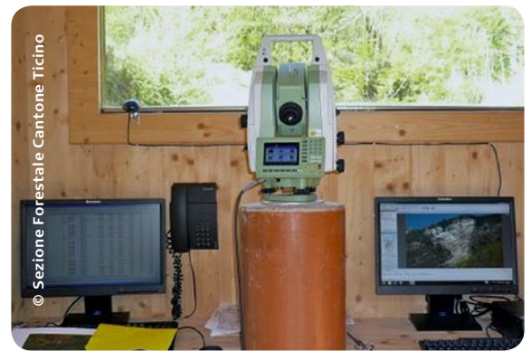
■ Leica TM30 monitoring the area.
