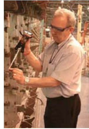
An Airbus employee uses the Leica T-probe to check assembly tooling.
