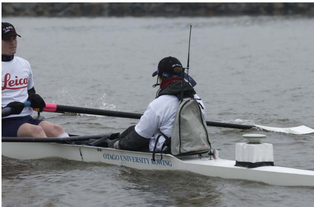
Figure 4: The location of the antenna on the stern of the men's eight.
