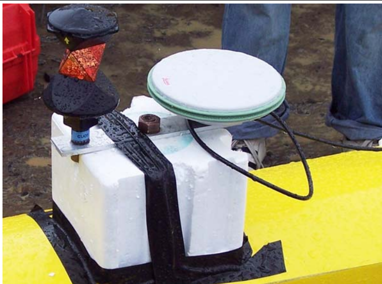
Figure 3: The polystyrene bracket used for mounting the GPS antenna and TPS 360 0 prism on the skiffs. The skiff shown is the Men's 1x
